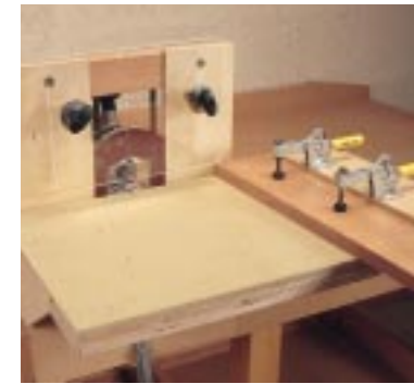
▶ A tube clamp bolted to the underside of the top, provides a stable mounting for the Trend Routerack overhead system. Various forms of back fence can then be cut from thick board or laminated sheet to suit specific operations, retained and adjusted by locking levers screwed into threaded inserts. Adjustable fence faces can be added to suit.
